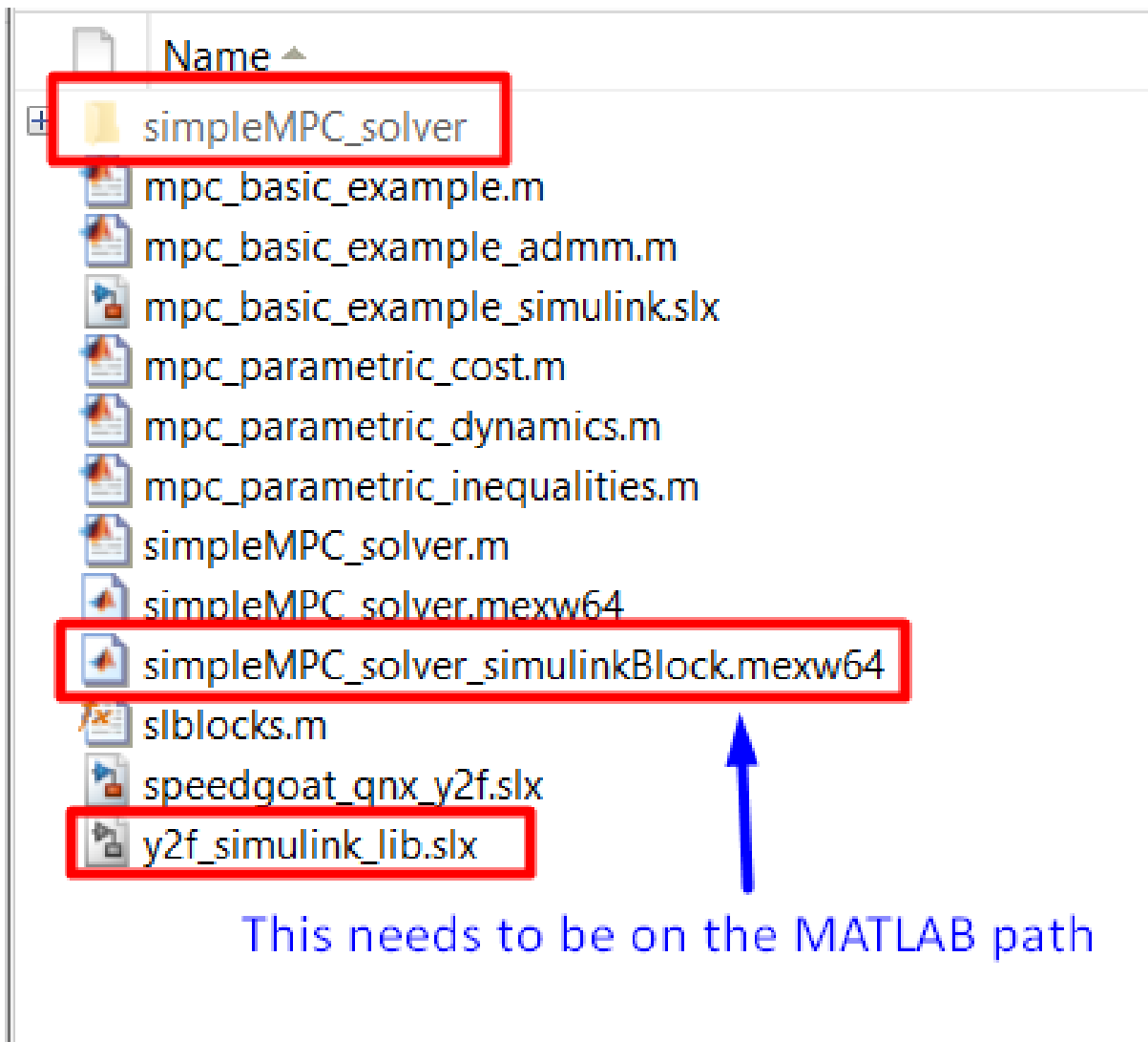
Figure 13.105: Add the folder containing the .mexw64 solver file to the MATLAB path.
